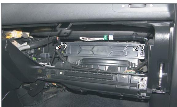
**EN** Remove the cover of the filter chamber, remove the old filter from the seat, put the new one in and perform the opposite to all the previous actions in the reverse order
