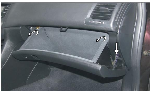
**EN** Remove the glove compartment
