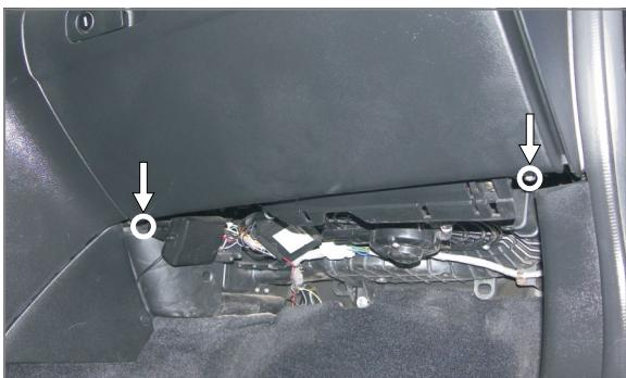
**EN** Unscrew the cover of the glove compartment
