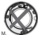
Connection of 100–240 V AC and 12 V DC must not be done simultaneously (Figure M).
