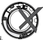
No 100–240 V cables may be laid over the electronics component (Figure N).
