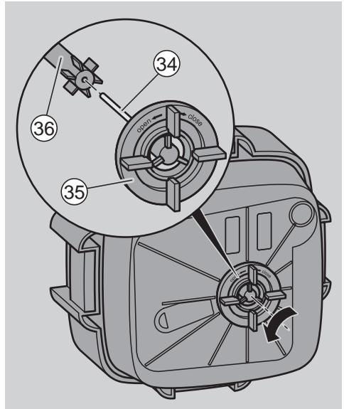
The impeller is on the bottom side of the motor head. The impeller is comprised of an impeller wheel (36) and an impeller shaft (34).
